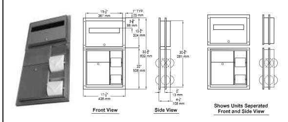
**MATERIALS:** The unit is fabricated of 18-8, type 304 stainless steel with a No. 4 satin finish and is one piece seamless 22 gauge flange construction.
