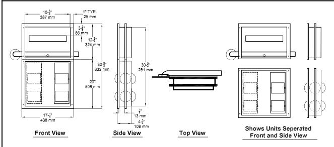
**MATERIALS:** The unit is fabricated of 18-8, type 304 stainless steel with a No. 4 satin finish and is one piece seamless 22 gauge flange construction.
