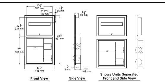
**MATERIALS:** The unit is fabricated of 18-8, type 304 stainless steel with a No. 4 satin finish and is one piece seamless 22 gauge flange construction.
