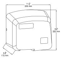
**SPECIFICATIONS:** Surface Mounted Automatic Touch Free Sensor Hand Dryer. 1/8 HP, 1800 Watts 110 Voltage/15 Amps and 220 Voltage/8 Amps. Cover is fabricated of one piece high grade fire retardant ABS, 3.0 mm thick, white color. 30-35 seconds drying time. Sound level is 55 ± 3dB. Dryer shall deliver 150 CFM, air speed 15.5 m/s. Weight is 8.4 lbs. (3.8 kgs). Drip Proof IPX1. Brushless motor 3150 R.P.M. The heater assembly is designed with 200° F (87 ° C) thermostat.
