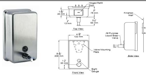
**MATERIALS:** 18-8 stainless steel, Type 304, 20 gauge dispenser. All exposed surfaces fabricated of No 4 satin finish. Valve constructed of chrome-plated brass body with stainless steel and plastic internal parts.
