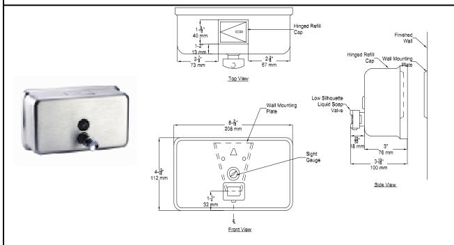
**MATERAILS:** Surface Mounted Horizontal Soap Dispenser fabricated of 20 gauge stainless steel, alloy 18-8, and type 304. All exposed surfaces fabricated of No 4 satin finish.
