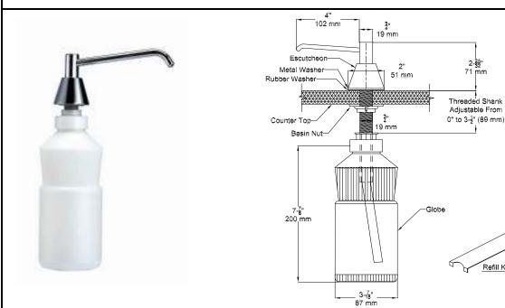
MATERIALS: 4" spout is stainless steel with rubber check valves and an O-ring seal. Valve body, internal parts, basin nut, threaded shank and globe adapter to be molded plastic. Spring, escutcheon washer, stem retainer collar and screw to be stainless steel. Escutcheon to be chrome plated brass, Soap container to be translucent, shatter resistant polyethylene.
