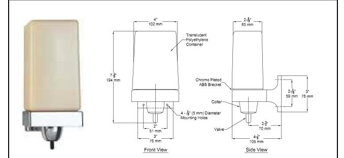
**MATERIALS:** (Push-up type) unit is fabricated of tamper resistant, chrome plated ABS plastic, a translucent white polyethylene soap container, and a corrosion resistant ABS dispensing valve with stainless steel spring.
