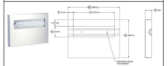
**MATERIALS:** The unit is fabricated of alloy 18-8 stainless steel, type 304, 22 gauge, with a No. 4 satin finish.
