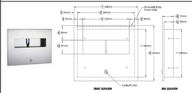
MATERIALS: The unit is fabricated of alloy 18-8 stainless steel, type 304, 22 gauge, with a No. 4 satin finish.
