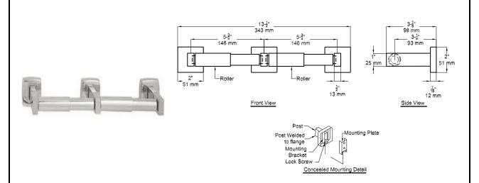
**MATERIALS:** Dual Roll Surface Mounted Toilet Paper Holder unit to be fabricated of 18-8 stainless steel type 304, satin finish. Posts to be fabricated of 1/2" x 1" (13mm x 25mm) rectangular tubes. Rollers to be chrome-plated high impact-resistant ABS plastic and two (2) shall be supplied
