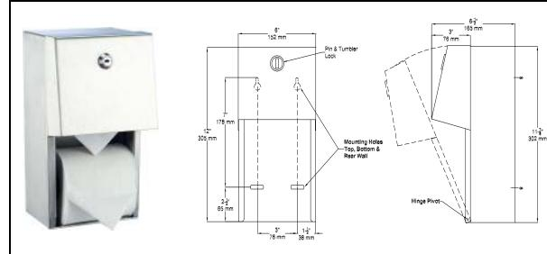
**MATERIALS:** Surface Mounted Toilet Tissue Dispenser fabricated of alloy 18-8 stainless steel, type 304, 18 gauge, cabinet body will be same grade, 22 gauge.
