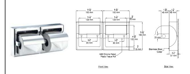
**MATERIALS:** 18-8 stainless steel, type 304, double roll holder with hoods and high impact resistant ABS plastic; chrome plated rollers.
