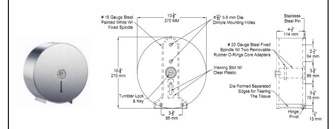
**MATERAILS:** Surface Mounted Jumbo Roll Toilet Paper Dispenser cover fabricated of alloy 18-8 stainless steel, type 304, 20 gauge with a No 4 satin finish. Cover will be of one piece construction hung on stainless steel pin hinges and will be held closed by a tumbler lock, key is provided.
