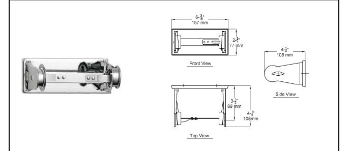
**MATERIALS:** Surface Mounted Single Roll Toilet Paper Holder to be fabricated of No18 gauge high polished chrome-plated steel.
