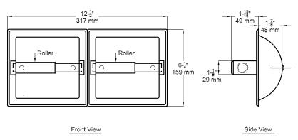
**MATERIALS:** Recessed Mounted Dual Roll Tissue Holder is fabricated of alloy 18-8 stainless steel, type 304. Rollers are fabricated of chrome plated, high impact resistant ABS plastic. Exposed surfaces have a bright finish.
