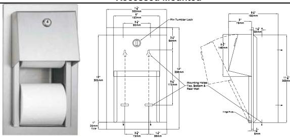
**MATERIALS:** 18-8 stainless steel, type 304, 18 gauge, door, door frame, and dispensing mechanism guide tracks fabricated; cabinet body to have same grade, 22 gauge. All exposed surfaces to be N<sub>o.</sub> 4 satin finish.
