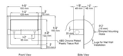
**MATERIALS:** 18-8 stainless steel, type 304, double toilet tissue roll holder with hood and high impact resistant ABS plastic; chrome plated roller. Exposed surfaces have a bright finish.
