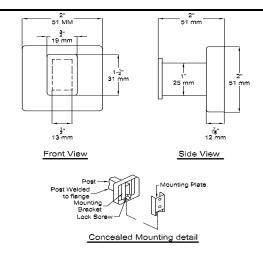
**MATERIALS:** Single Robe Hook to be fabricated of stainless steel alloy 18-8, type 304.
