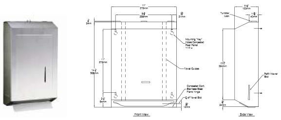
**MATERIALS:** The surface mounted paper towel dispenser is fabricated of 22 gauge, type 304 stainless steel alloy 18-8, with No. 4 satin finish.
