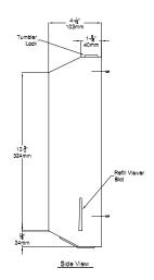
**MATERIALS:** The surface mounted towel dispenser is fabricated of white steel and fitted with tumbler lock and heavy duty steel piano hinge.
