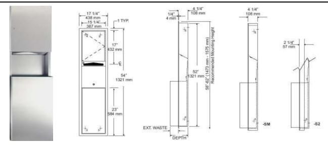
**MATERIALS:** Towel dispenser, door, frame, waste container and cabinet shall be fabricated of alloy 18-8 stainless steel, type 304, 22 gauge All exposed surfaces to be No. 4 satin finish.
