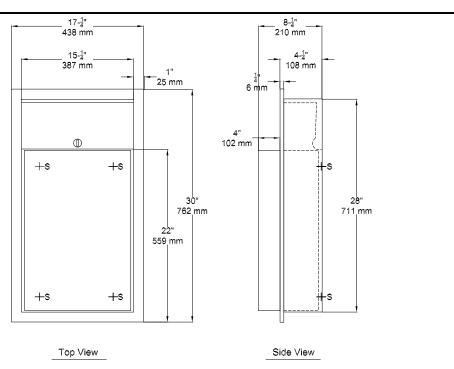
MATERIALS: The unit is fabricated of 22 gauge, type 304 stainless steel, No.4 satin finish.
